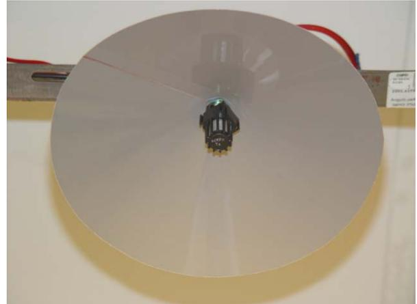
Fig. 6. Aspect of the prototype: cylindrical PVDF transducer with conic reflector.
