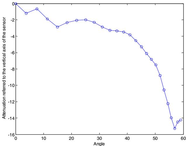
Fig. 10. Attenuation referred to the vertical axis of the sensor, determined by experimental measurements.
