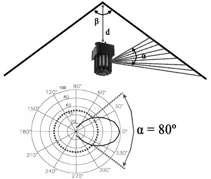
Fig. 3. Position of the transducer inside the conic reflector and vertical beam directivity of the transducer.
