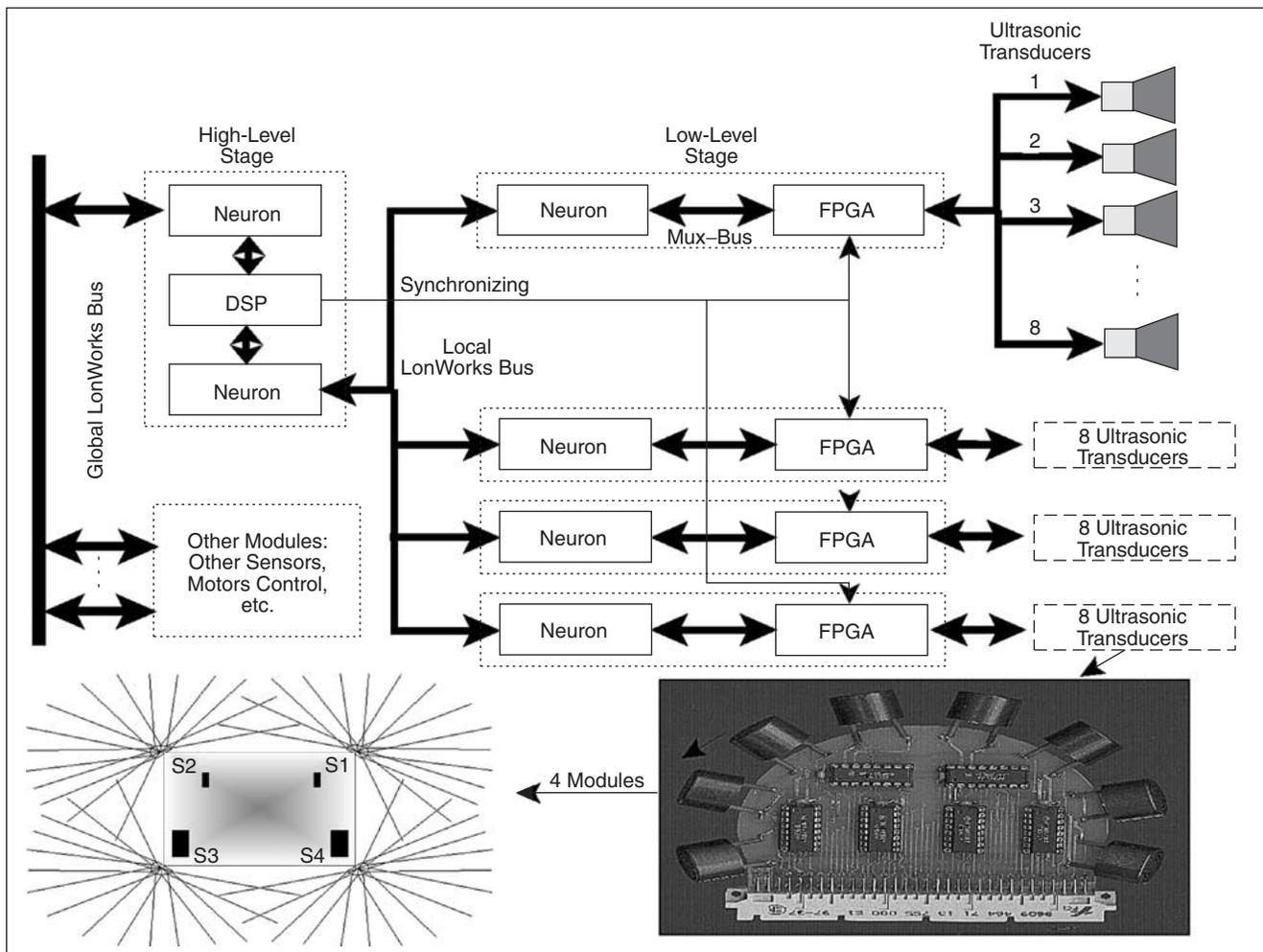
Fig. 5. Block diagram of the ultrasonic system.
