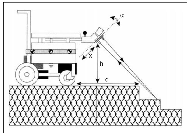
Fig. 6. IRED and PSD configuration on the wheelchair.
