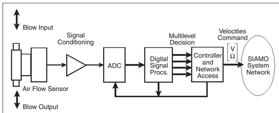
Fig. 2. Block diagram of the breath-expulsion unit.
