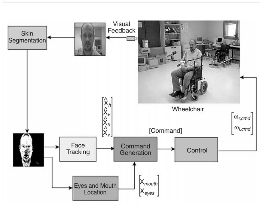
Fig. 3. Architecture of guidance by head movements.
