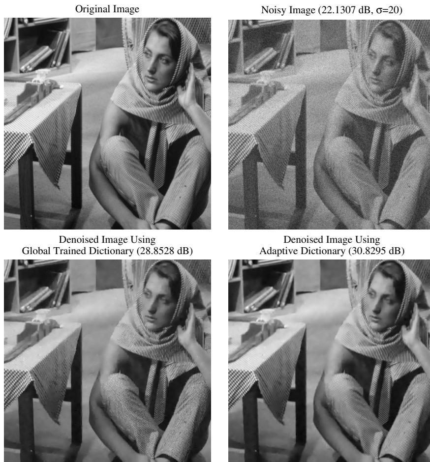
Fig. 10 Denoising comparisons: Additive noise standard deviation \sigma = 20 ; i.e., unprocessed PSNR = 22.13dB. The results using the globally trained and the adapted K-SVD dictionaries with patches of 8 \times 8 show an improvement of 6.7 and 8.7dB, respectively.
