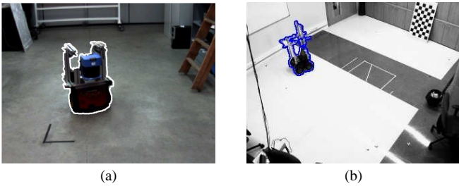
(a) (b) Fig. 8. Initial curves obtained after removing the shadows (a) Image 120 of the sequence 1 (Fig. 6.a) (b) Image 250 of the sequence 2 (Fig. 6.b)
