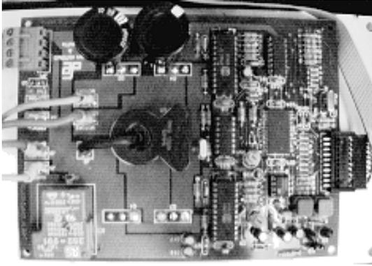
Figure 7.- DC-motor board, with the controller, drivers and H-bridge.
