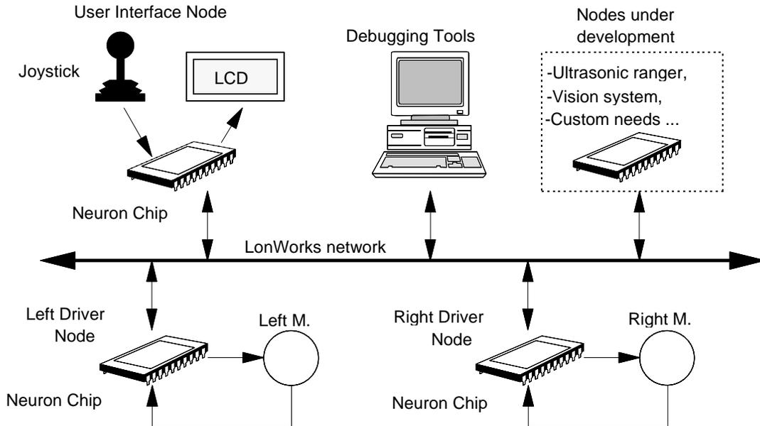
Figure 5.- Block diagram of the Wheelchair.
