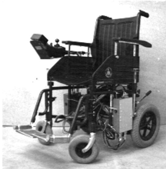
Figure 8.- Wheelchair with Lonworks architecture.
