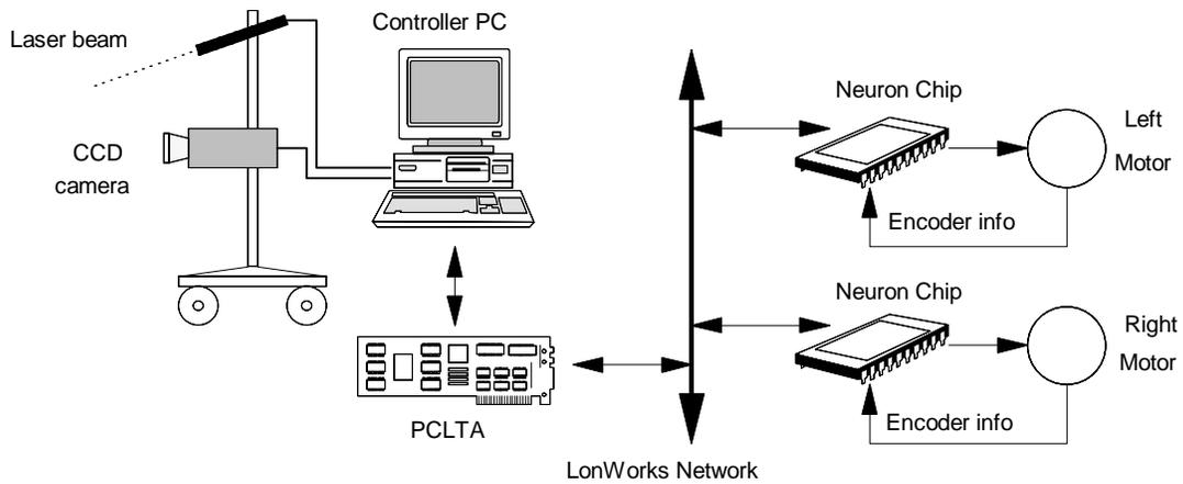
Figure 4.- Diagram of the Mobile Robot, guided by a laser range finder.
