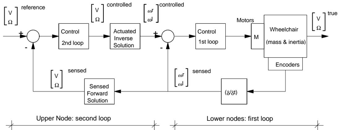
Figure 6.- Double control loop in the Wheelchair.
