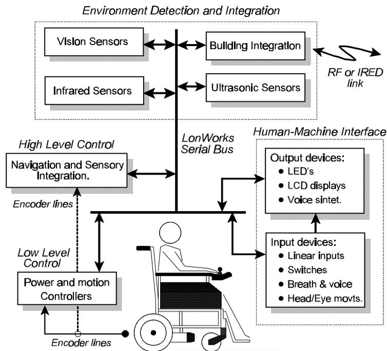
Figure 1.-SIAMO system, functional diagram.
